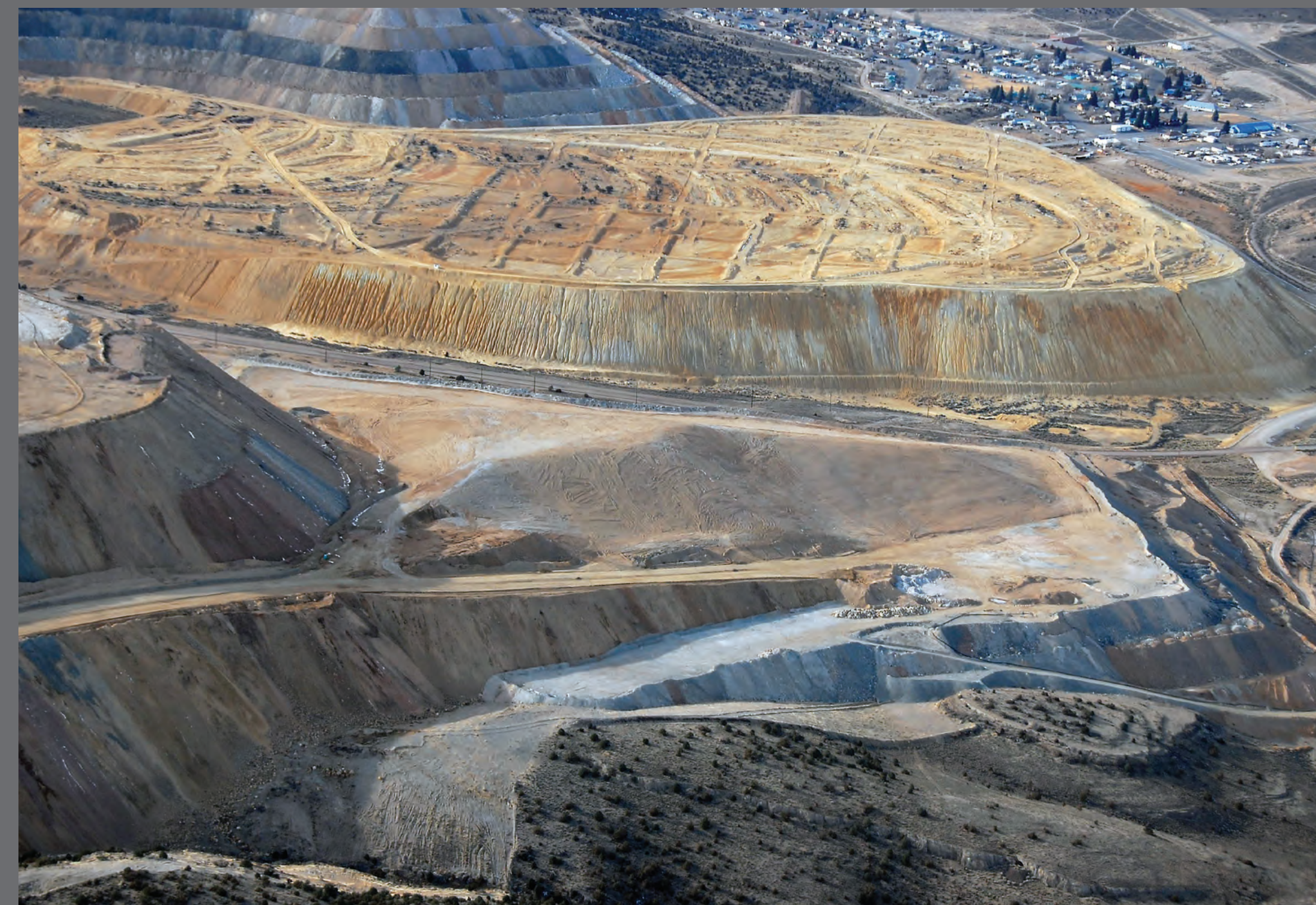
LEACHING COPPER AT KEYSTONE DUMP The town of Ruth at upper right is dwarfed by Keystone Dump in this 2018 aerial view. The grid patterns on the dump are leaching pond berms. Beginning in 1919, Ruth mining companies leached small but profitable amounts of extra copper by slowly flowing water through the Liberty Pit dumps, collecting the fluid, sprinkling it over scrap metal, and recovering the precipitated metallic copper. Leaching at Keystone was less successful than at the Mollie Gibson, Puritan, and Sunshine dumps, and ended in 1949. Source: KGHM Robinson Nevada Mining
