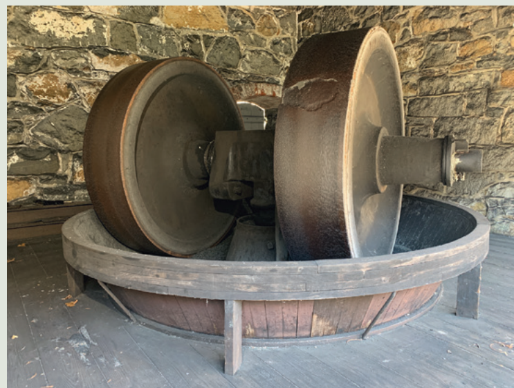
A typical gunpowder "wheel mill" had two heavy rotating wheels that turned in a round pan to grind the ingredients to a fine powder. Source: Hagley Museum & Library
