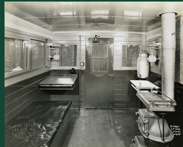
◀ SPARTAN INTERIOR A 1942 photograph of a New Haven Railroad caboose shows a bunk, conductor's desk, canteen, sink, and stove with railings to keep pots from sliding off when the train was moving. Source: David Peters Collection / Archives & Special Collections, UConn Library.
