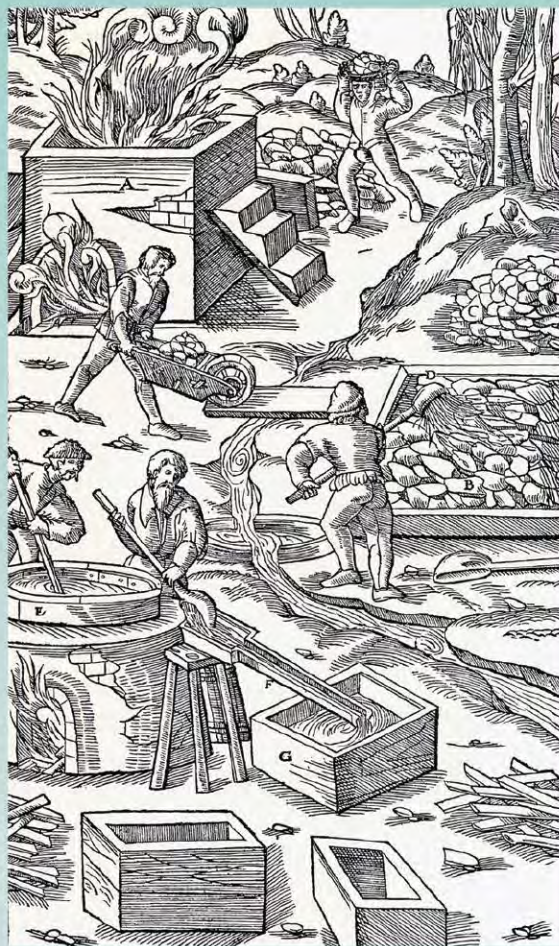
A sixteenth-century German print showing key copperas-making steps. At top, a miner carries ore to a chamber for roasting. At center, miners move roasted ore to a leaching heap and sprinkle water on it to make weak copperas liquor. At bottom they concentrate the liquor in a boiler and tap it into a vat to cool and settle before crystallizing. Source: Georgius Agricola, De Re Metallica, 1556. Dover Publications Inc.
