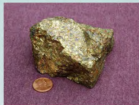
Sample of chalcopyrite (copper sulfide ore) mined underground at the Elizabeth Mine. Source: U.S. Environmental Protection Agency.
