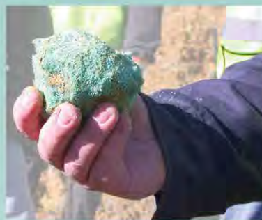
Naturally formed weak copperas found in waste material at the copperas works area before the Superfund cleanup. Water runoff from the area included acid and metals generated by this kind of mine waste. Source: U.S. Environmental Protection Agency.
