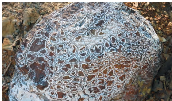
Weak white iron sulfate (copperas) coating forming naturally on a lump of pyrrhotite (iron sulfide) ore, Elizabeth Mine, South Strafford, Vermont. Source: U.S. Environmental Protection Agency.
