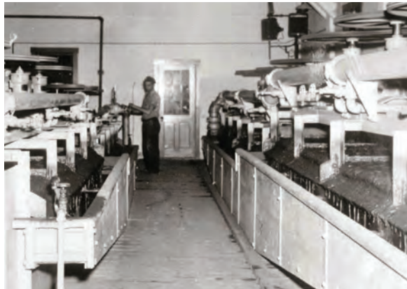
Froth flotation tanks in the flotation mill, 1950s. The dark foam dripping off the top of the tanks is finely ground copper ore that has been attracted to chemical bubbles. Source: Strafford Historical Society.
