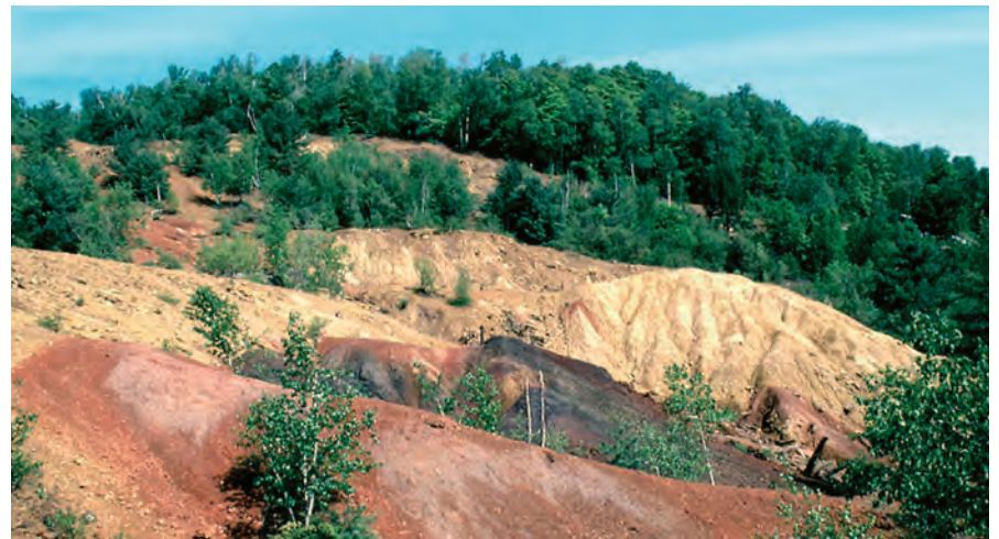
Eroded copperas manufacturing roast beds / heap leach piles on Copperas Hill. The leachate from this area produced copper concentrations in Copperas Brook over 5,000 times greater than the Vermont water quality standard of 11.8 parts per billion.
