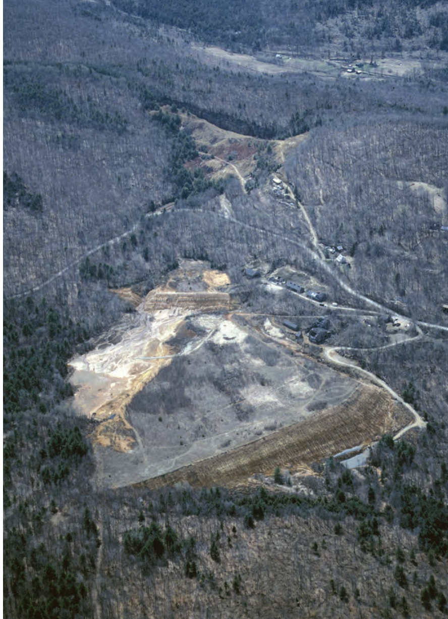
Aerial view looking southwest in 2003 showing ore mill tailings at center, World War II-era buildings at center right, Mine Road above and copperas works area with North Open Cut near top. Hillside topography funneled surface and groundwater through the site, gathering acid and metals and carrying them north into the Ompompanoosuc River. Source: U.S. Environmental Protection Agency.
