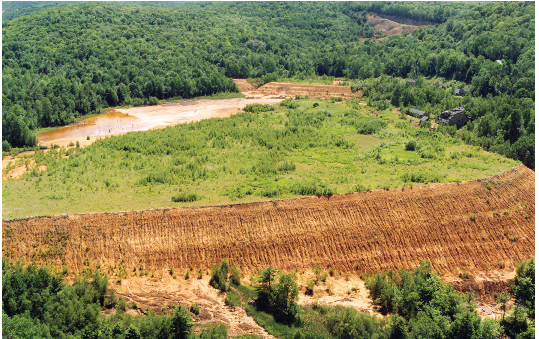
Aerial view of partially overgrown copper ore mill waste tailings pile in Copperas Brook valley looking southwest, 1990s. Copper ore was processed and separated from the tailings in the mill buildings at center right, 1943–1958. About 2.8 million cubic yards of tailings were discarded in the 45-acre pile, which is a quarter of a mile wide on its 150-foot-high north face. The North Open Cut and copperas works area are visible at upper right. Source: Strafford Historical Society.
