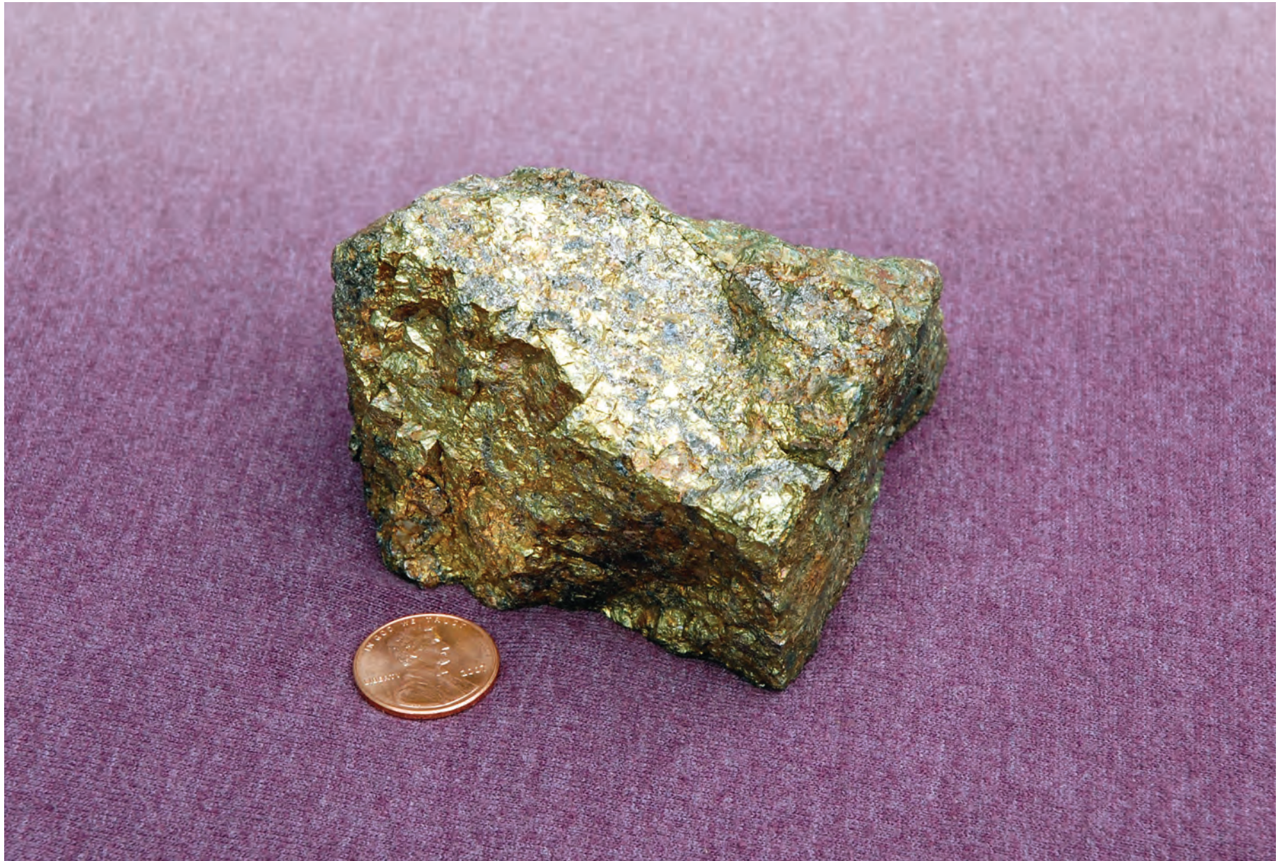
Sample of chalcopyrite (copper iron sulfide) ore taken from underground at the Elizabeth Mine in the 1950s, with copper penny for scale. Source: Matt Kierstead.
