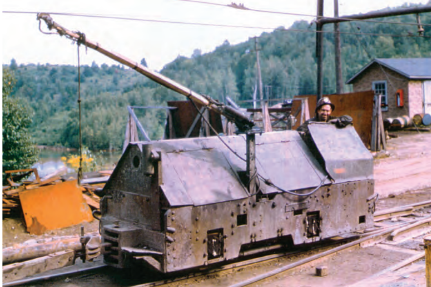
A miner poses with an electric mine locomotive, which is protected from falling rocks by the sheet metal cover, 1950s. Source: Strafford Historical Society.
