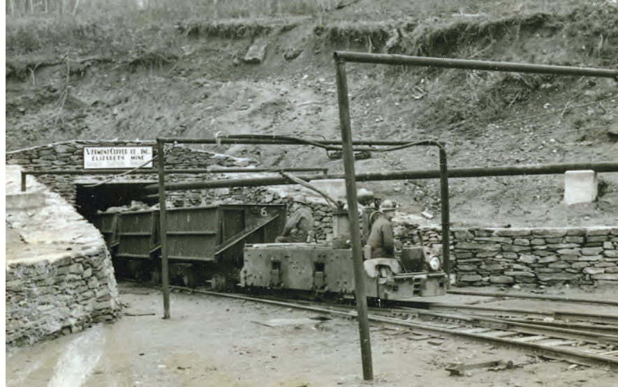
An electric mine locomotive exits the 1898 adit with a load of copper ore for the mill, sometime during the 1950s. Mine locomotives took electricity off an overhead trolley wire. Source: Strafford Historical Society.
